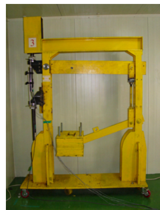
Fig. 2 Creep test device for GFRP rebar
