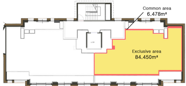
Figure 4. Apartment Area Calculation Range Using Revit2013
