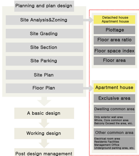
Figure 3. Area Calculation in Housing and Apart
