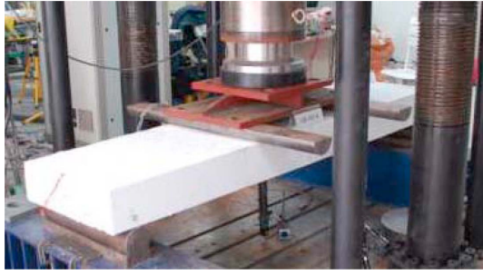
Fig. 2. 4-points bending test.
