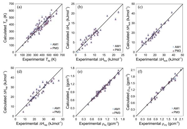
**Figure 1.** Plots of calculated *vs* experimental values computed using semi-empirical methods. (a) Normal boiling points, (b) Heats of fusion, (c) Heats of sublimation, (d) Heats of vaporization, (e) liquid density, and (f) crystal density.
