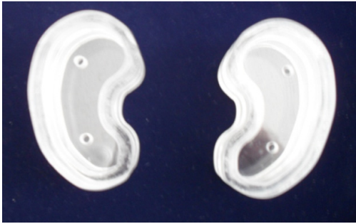
Fig. 2. It has devised in completion of acrylic phantom and outlet & inlet.
