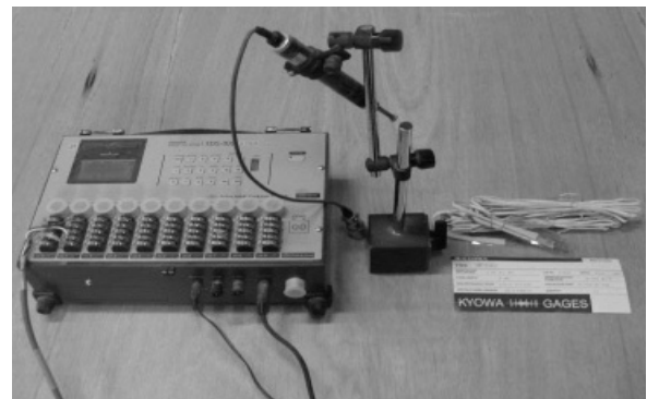
Fig. 6. Data Logger, LVDT and Triaxial gauge
