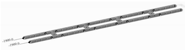
Fig. 6. Finite element modeling of the PCT test specimen
