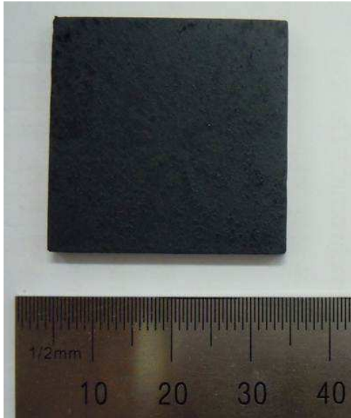
Fig. 2 LSMO sample using sol-gel method and spin coating
