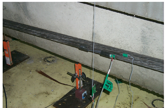
Fig. 4 Figure of repaired test member by epoxy (CR1H)
