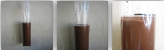
Photo 2 Bleeding test method
