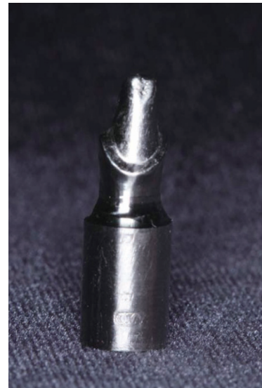
Fig. 1. The metal die used for the fracture strength test.
