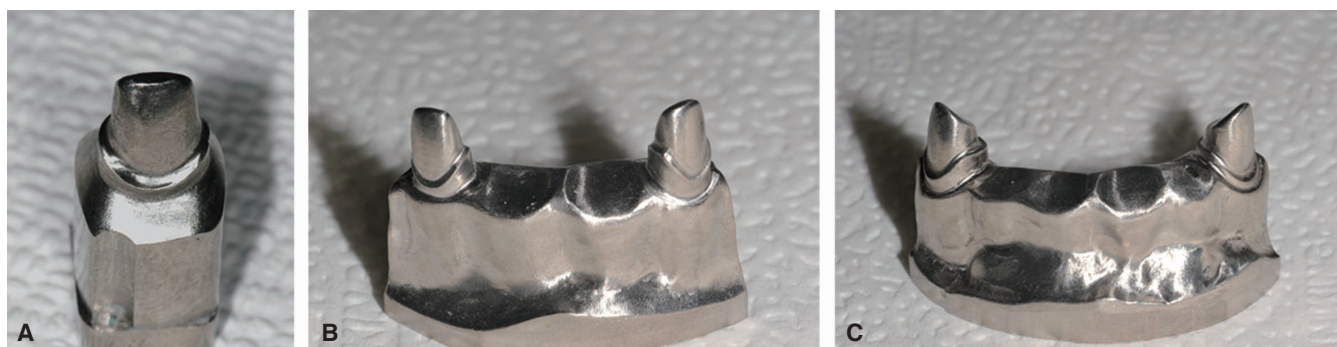
Fig. 1. Titanium master model fabricated using CAD/CAM (Addtech Co., Seoul, Korea). A: single, B: 4-unit, C: 6-unit.
