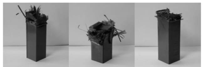
Fig. 5 Shapes of Collapsed CFRP Square member (Impact energy 372 J)
