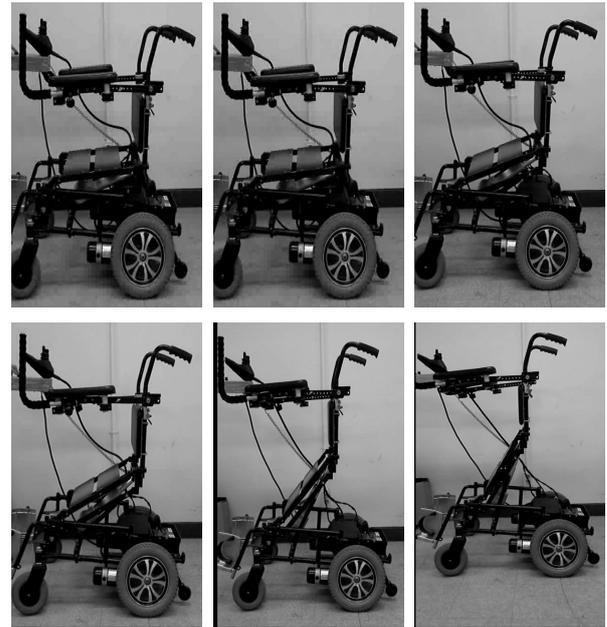
**Fig. 8 Lift motion of wheelchair**
