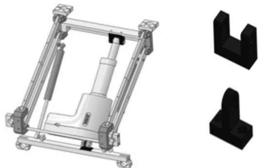
Fig. 6 Upper and lower bracket for linear actuator
