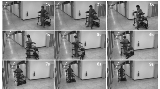
Fig. 15 Snapshots of forward and right turning walking test
