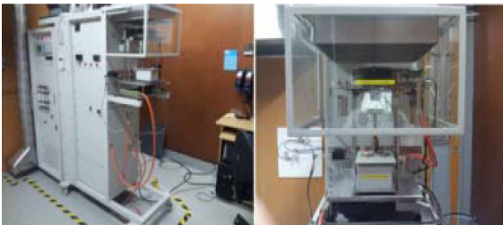
Fig. 9. Cone calorimeter test.
