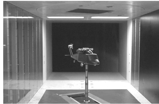
Fig. 3. Fuselage drag-stability model[9]
