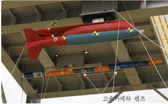
Fig. 4. Installation of Gliding Bomb and Camera Pod Under Test Bench
