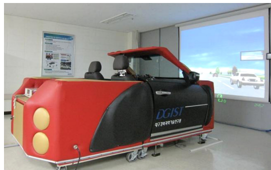
Fig. 1 DGIST Fixed-base driving simulator
