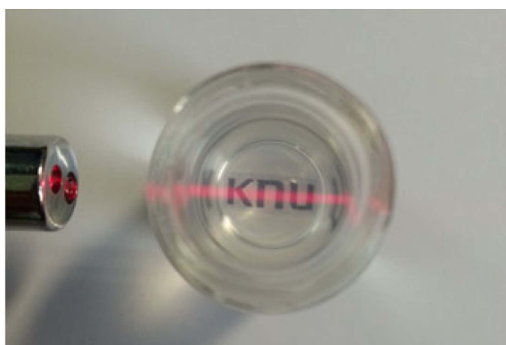
Figure 3. Tyndall scattering from exfoliated perovskite colloidal suspension.
