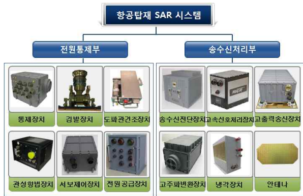
Fig. 1. Configuration of airborne SAR system
