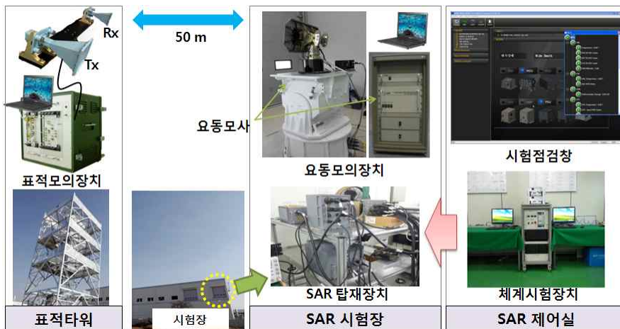
Fig. 7. Configuration for ground test
