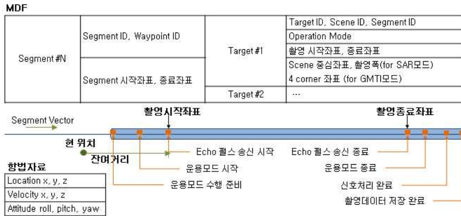
Fig. 5. Operation mode execution concept based on MDF
