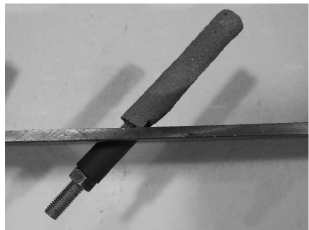
Fig. 2. Model bolts installation
