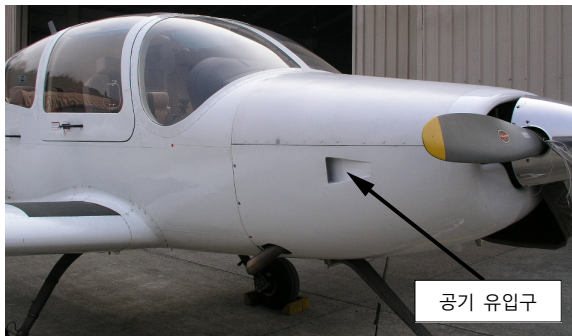
Fig. 2. Air inlet of T-103
