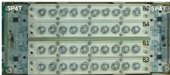
Fig. 16. A fabricated filter bank
