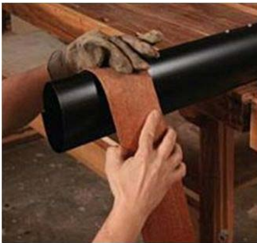
Fig. 6. Hot-plate heating bent wood.
