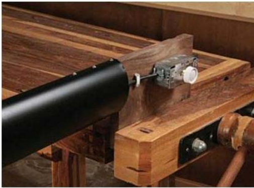
Fig. 5. Hot-plate heating bent wood.
