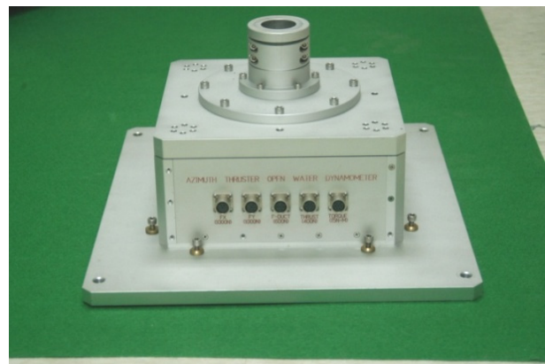
Fig. 8 Multi-component force sensor for measuring total thrust and other components
