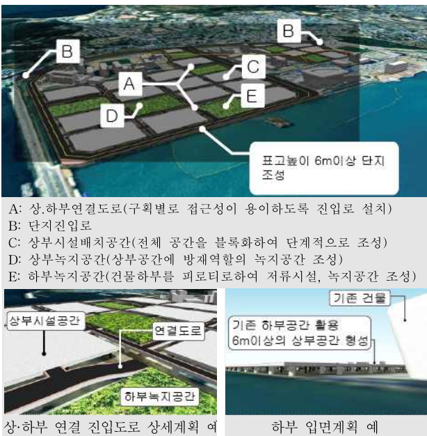
Fig. 11 Steps for flooding prevention at reclaimed area
