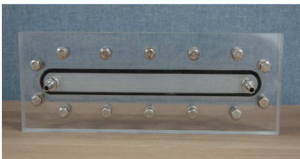
Fig. 2 Prototype of planar membrane humidifier
