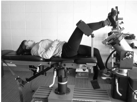
Figure 1. Starting position for measurement using isokinetic dynamometer.
