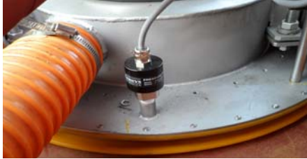
Figure 8: Pressure sensor on the adhesive pad
