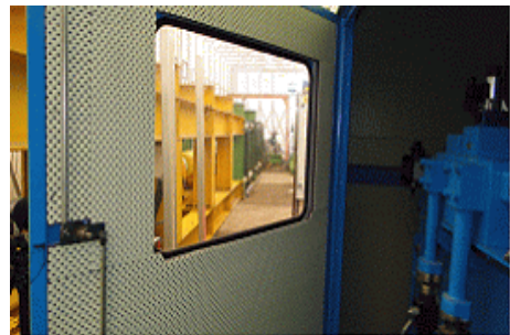
Figure 5: Internal feature of shield chamber covered by sound-absorbing materials
