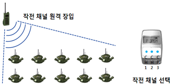
Fig. 8. Communication security using channel selection
