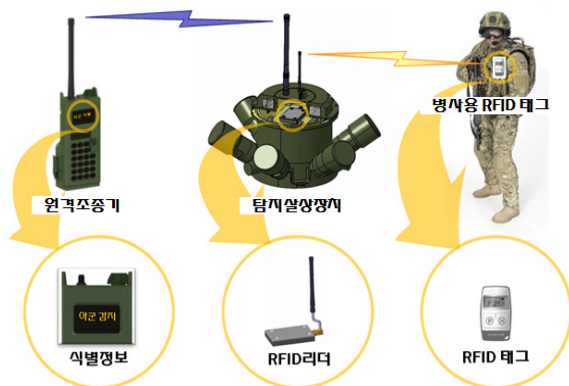
Fig. 1. System block of IFF landmine
