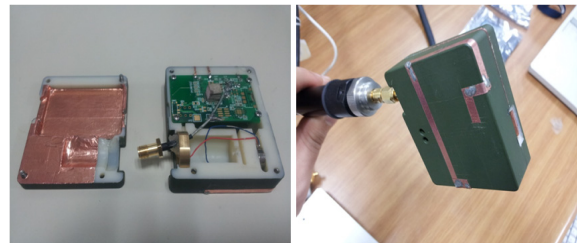
Fig. 12. Antenna design revision of RFID tag
