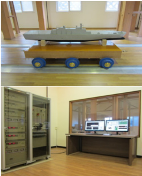
Fig. 8. Magnetic field measurement test using scaled model ship
