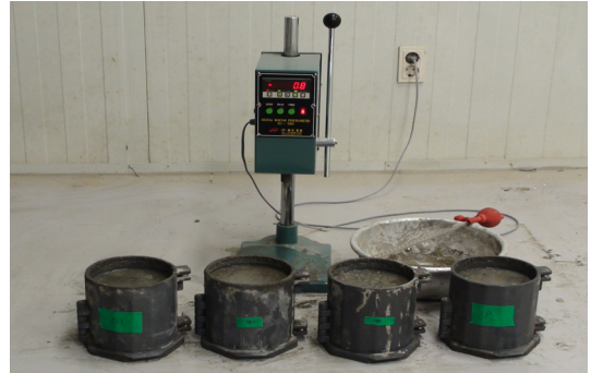
[Fig. 2] Testing method for time of setting of concrete mixture by penetration resistance
