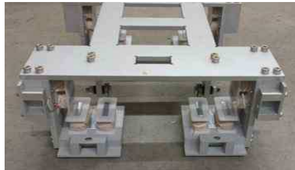
Fig. 4. The picture of the quadruple hybrid EMS system which was actually used for experiment
