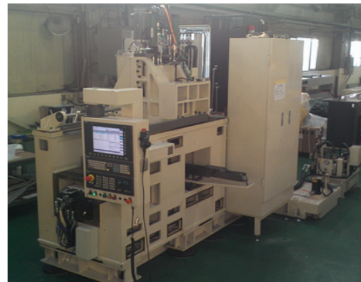
Fig. 15 The picture of Vertical Grinding System
