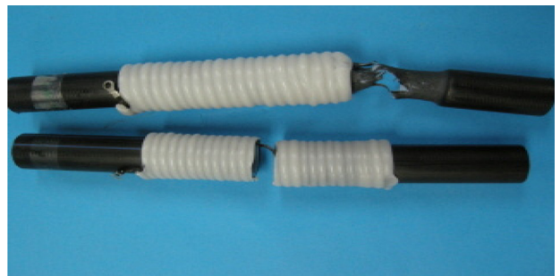
Fig. 6 Fracture at pipe(top) and fracture at socket-pipe(bottom)
