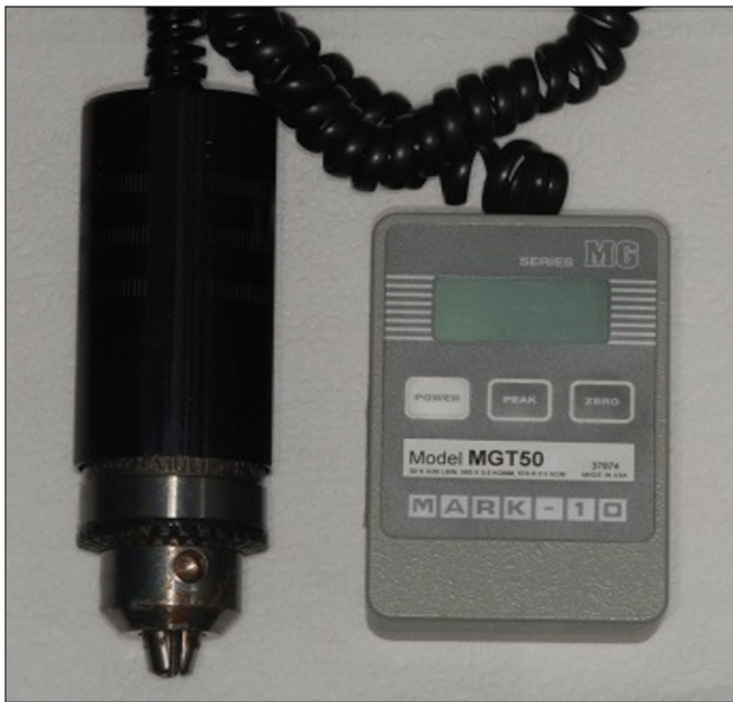
Fig. 3. Digital torque gauge (MGT50) was used to tighten the abutment into implant at desired torque.
