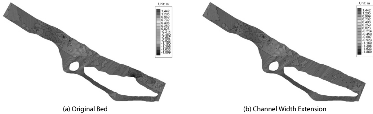
Fig. 11. Bed Change Comparison after 30 Days ( Q = 1,000 \text{ m}^3/\text{s} )
