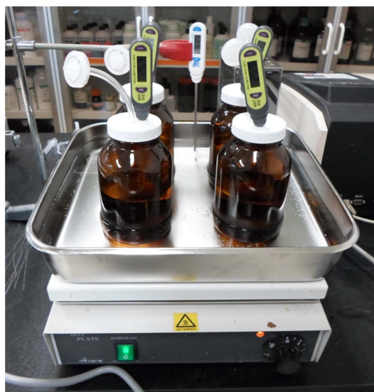
Fig. 1. Lab-scale experimental of heating treatment for DNAPL groundwater.
