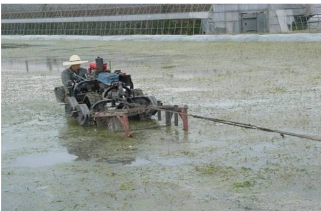
Figure 11. View of drawbar pull test of the prototype crawler vehicle.
