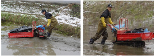
Figure 7. View of the driving test for the test crawler vehicle.
