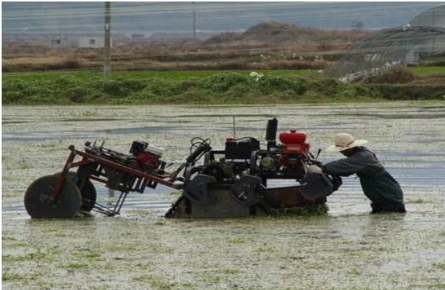
Figure 10. View of driving test of the prototype crawler vehicle.
