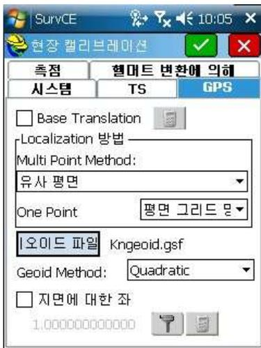
Figure 3. Realtime conversion of ellipsoid height to elevation using KNGeoid13 Geoid model
