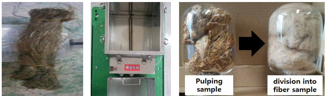
Fig. 1. The pulping machine for scouring of ramie material and ramie fiber.
