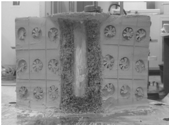
Fig. 11. Shear strength measuring locations (OD-150)
