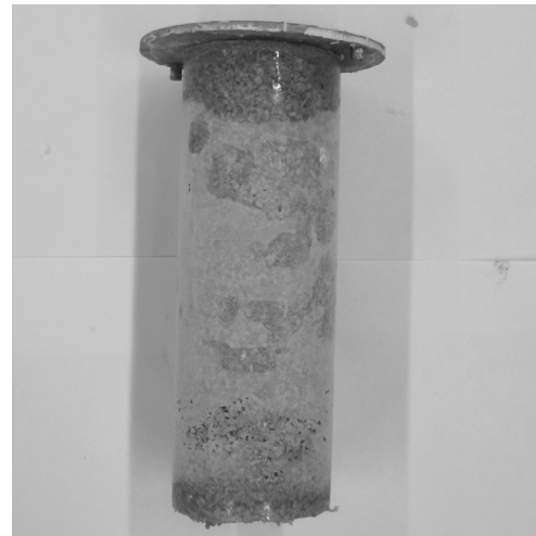
Fig. 4. Frozen reactive drain pile
