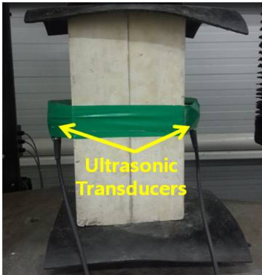
Fig. 1 Test specimen with ultrasonic transducers
