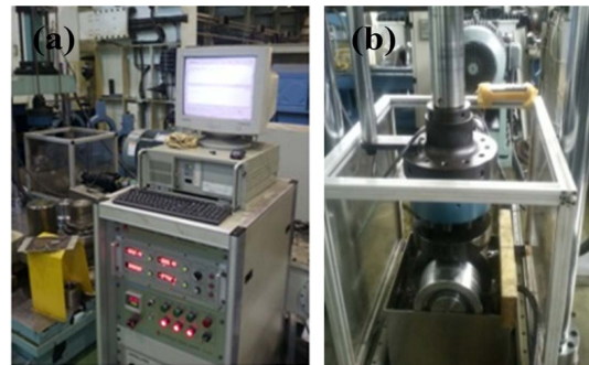
Fig. 9. Appearance of bearing control board (a) and durability tester (b).
