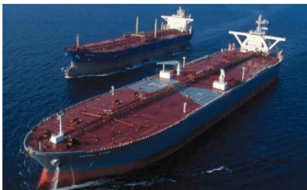
Fig. 1 Two tankers coming alongside in open waters to commence cargo transfer (The forward speed during the approach is in the range of 4-6 knots according to A courtesy of SPT Ltd.)
