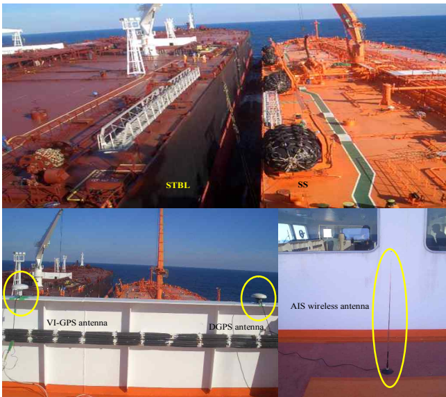
Fig. 4 Final stage of STS lightering between STBL and SS (top), GPS antennas (bottom left) and AIS wireless antenna (bottom right) installed on the wing bridge of the SS carried out in Gulf of Mexico
