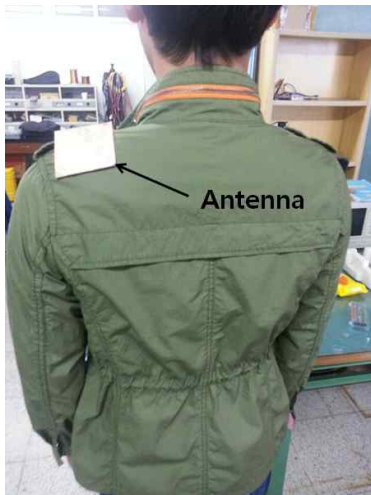
Fig. 8 Configuration of antenna integrated on cloth
