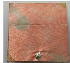
Fig. 6 Fabricated GPS wearable antenna
