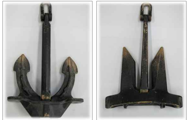
Fig. 1 ASS(left) and AC-14(right) type model anchor
