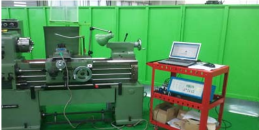
(b) 2D cutting test equipment
